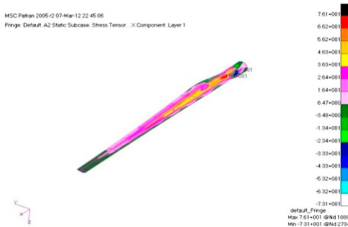
Figure 17. Spanwise stress contour on spar (21th ply) due to type II fatigue loads.
